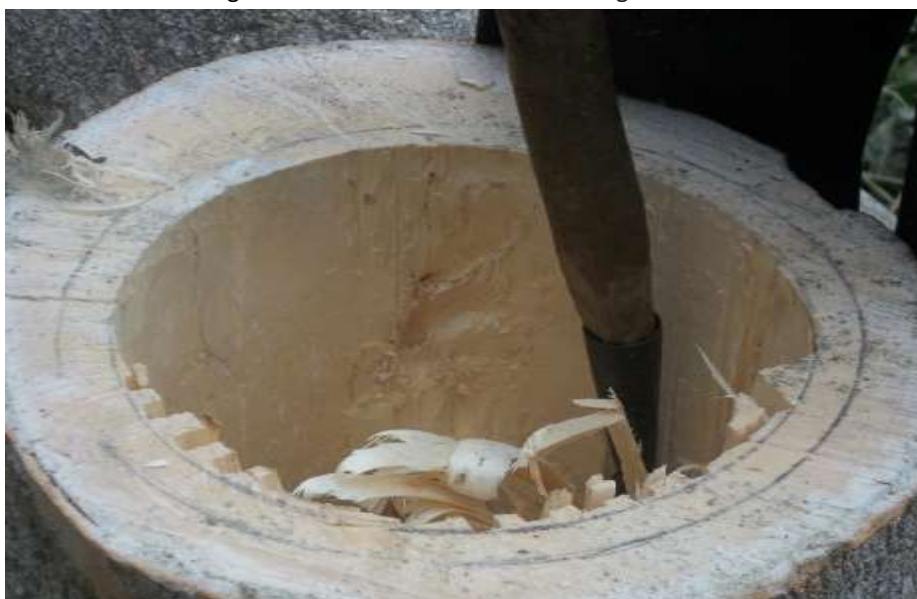
Figur 5. The process of cleaning the inside to form a tube
