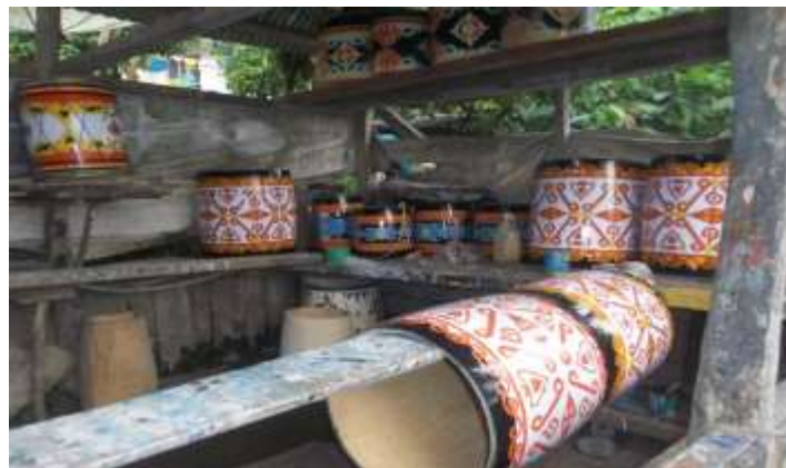
Figur. 10 The process of drying the Tambu drum after it has been colored
